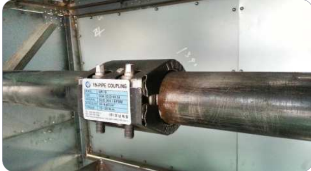
▲ The product just before the fire test, after being installed in a furnace
