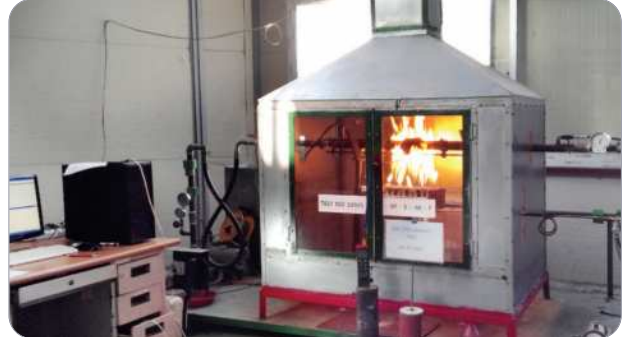
▲ The product during the fire test according to ISO 19922 regulation
